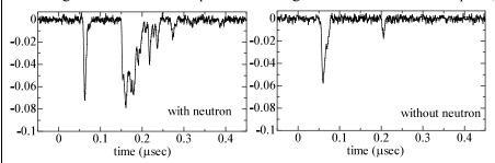
Even when neutrons are not applied (right), two peaks are often observed. They are attributed to photons directly from remaining 532 nm laser pulse and from delayed 905 nm
