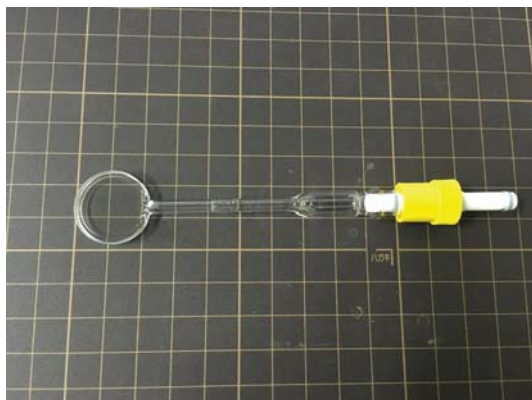
Figure 1. A quartz cell with a high vacuum greaseless stopcock. The path length was 2.0 mm.
