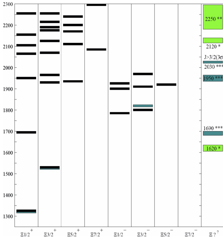
FIG. 1. Black bars: Predicted \Xi spectrum based on the quark model calculation [3]. Colored bars: Observed states. The two ground states and \Xi(1820) are shown in the column of J^P = 1/2^+, 2/3^- , respectively. Other unknown J^P states are plotted in the rightest column. The number represents the mass and the size of the box corresponds to the width of each state.
