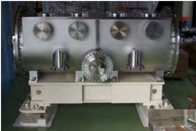
Vacuum chamber of the new injection-kicker magnet (above); Mount for the new magnet (right)
