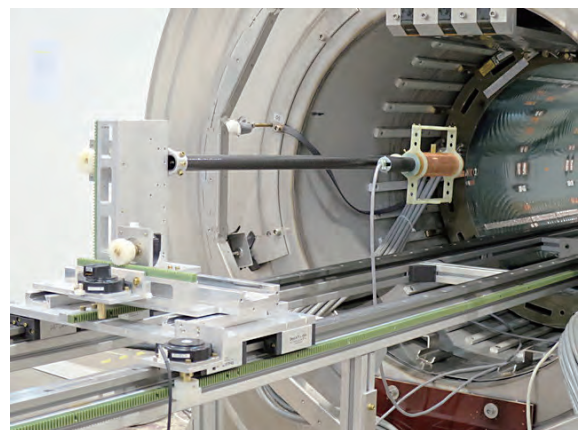
Fig. 6. The standard probe developed in KEK, tested with the MRI magnet at ANL.
