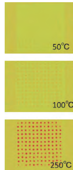
Fig. 6. Thermal image obtained with infrared bundled hollow-core fibers with 12 by 12 channels for profile monitor at the TEF-T.
