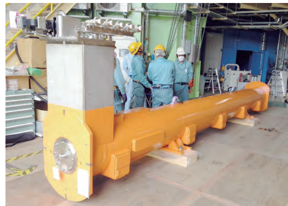
Fig. 4. A new superconducting solenoid with a warm bore for the MUSE D-line.
