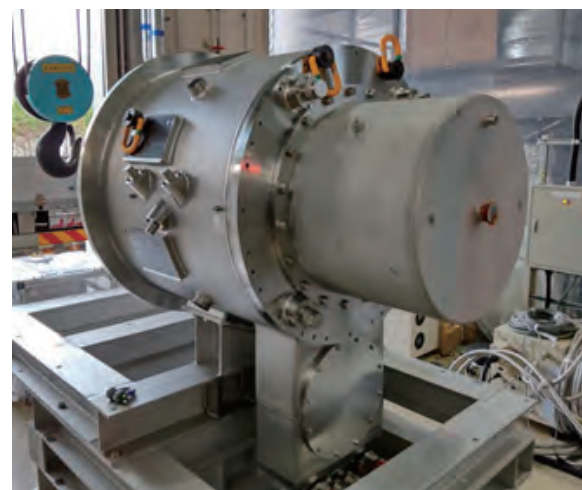
Fig. 6. Picture of the Bridge Solenoid delivered at J-PARC
