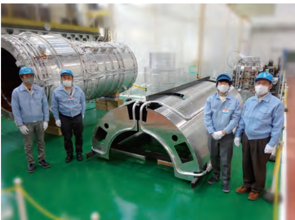
Fig. 5. Photograph of the fabricated cold masses and thermal shields of the PCS.
