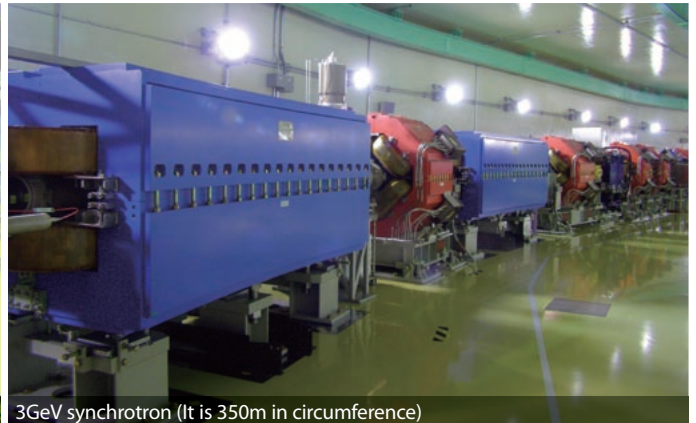
3GeV synchrotron (It is 350m in circumference)
